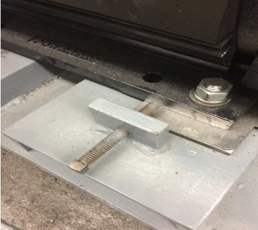
FIGURE 12: CAPS MOTOR TEST RIG HORIZAONTAL SET SCREWS
